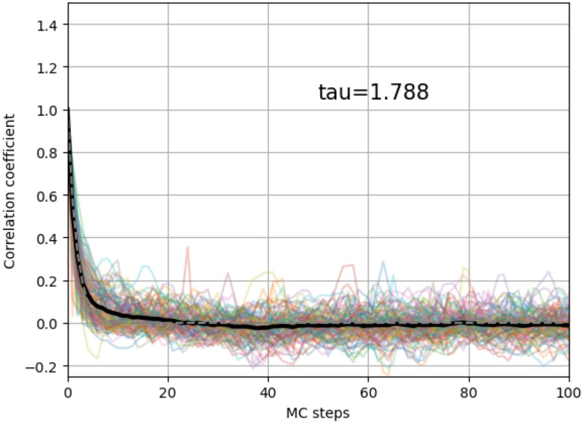
On this picture is represented the autocorrelation coefficient of the local energy of all the walkers (transparent colorful line) and the average of the autocorrelation coefficient (thick black line). This mean value is fitted with an exponential decay to obtain the autocorrelation time that is here equal to 1.79 MCs.
